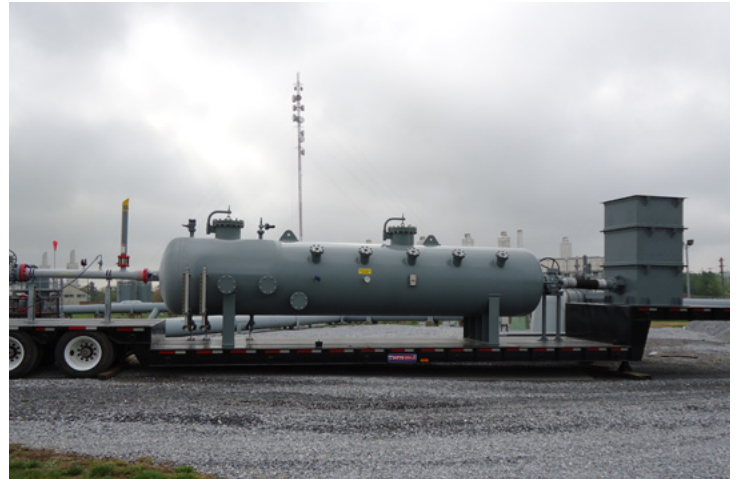
A mobile pipeline pigging system featuring a trailer mounted KLS separator and large carbon bed deodorizer integrated in one horizontal vessel, plus an HVVS vent silencer (right).
